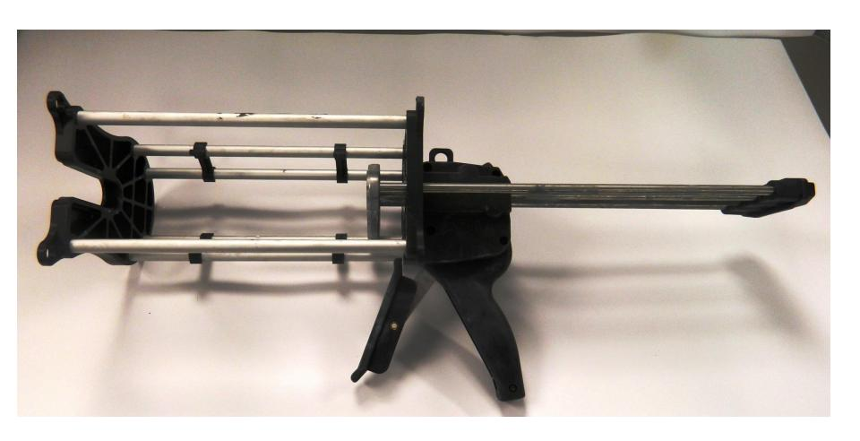
IT IS DESIGNED TO EXTRUDE PRODUCT THROUGH A STATIC MIXER, AND IS <u>INCAPABLE</u> OF SPRAYING ARC COATINGS
